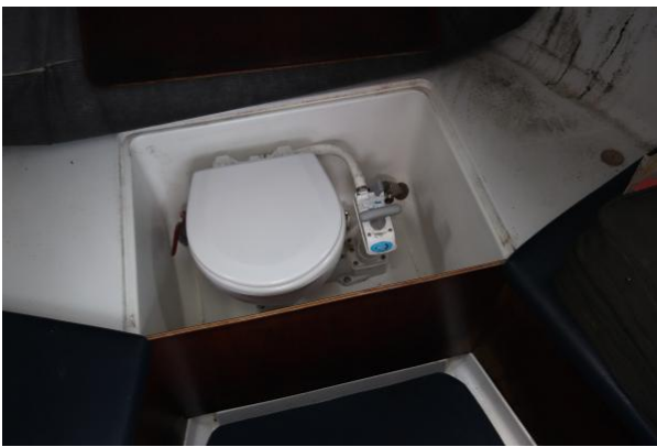
Beneteau Antares 620 sea toilet under foreberth
