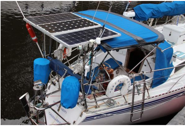
Gitana 43 gas bottles and solar panels
