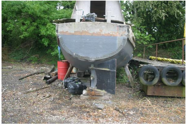
Naval Pinnace wooden hull sheathed
