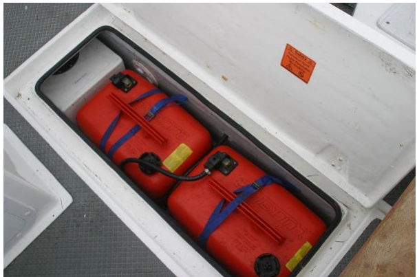
Nord Fisher fuel tanks
