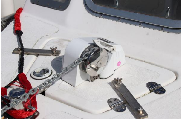
Nord Fisher electric anchor windlass
